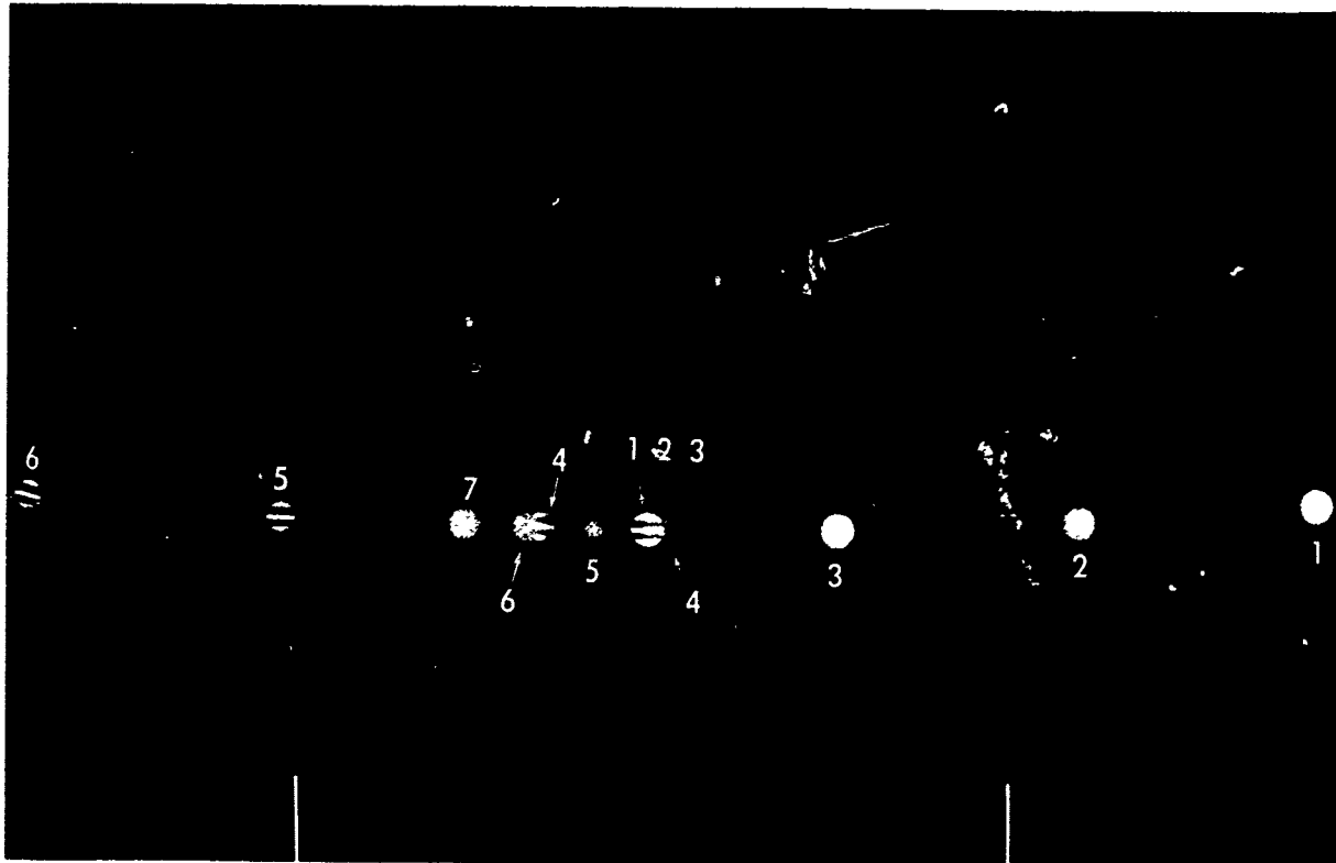
Figure 3. Stroboscopic photograph of Event 1. 10 flashes per second. The numbers shown do not appear in the photograph given to the student. They correspond to the order in which the successive flashes occurred at 1/10 second intervals. Each position of each ball can be associated with one of these numbers. The centers of the tops of the 2 rods appearing near the bottom of the picture are 1 meter apart and serve as a scale reference. (Available as a transparency.)
